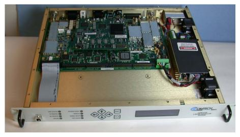
Figure 1. MPP70 correctly installed in the CDM-570L modem
