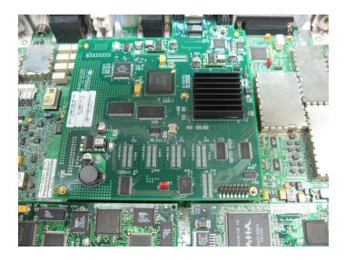
Figure 5. MPP70 board correctly installed in the CDM-570L modem
