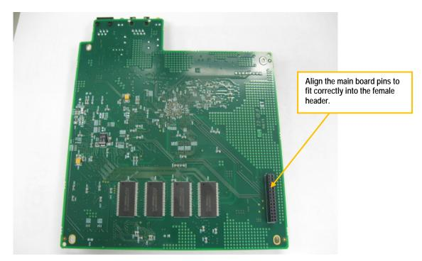
Figure 3. MPP70 Bottom side view
