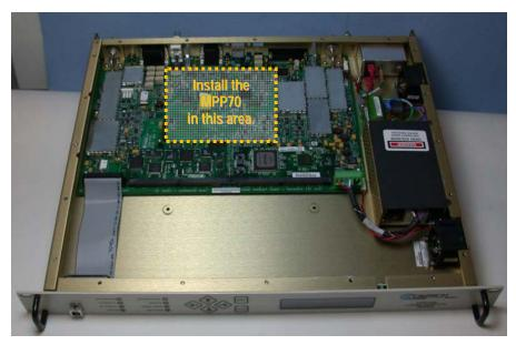
Figure 2. MPP70 properly installed in the CDM-570L modem
